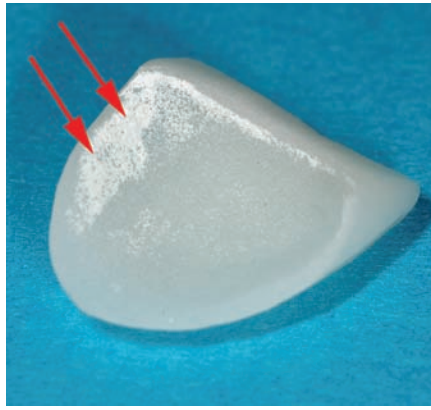
FIGURE 2 In this example, the intaglio surface of a porcelain veneer was purposely over-etched by the author with 9.5% HF placed for 15 minutes. Much of the clearly visible “white residue,” a combination of porcelain salts and porcelain debris, could not be removed even after an aggressive air/water spray for two minutes and wiping with cotton pellets soaked in acetone.
