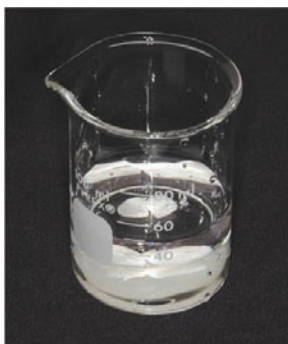
FIGURES 3A THROUGH 3C A useful technique for cleaning veneers is to place them in ethanol followed by ultrasonication. In this case, a full 15 minutes of ultrasonication was required to remove the white residue on the veneer depicted in Figure 2.
